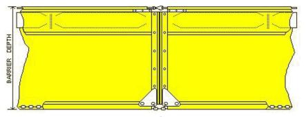
Type 2.DOT is the work horse of the TOUGH  $GUY^{(R)}$  line. It has a top load cable and special stress plates for reinforcing the corners and is designed to handle more severe conditions. It is recommended for lakes, streams, intercoastal and tidal areas where current velocities up to five feet per second are expected.
