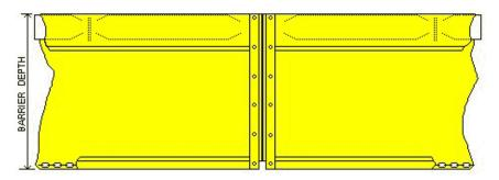
Type 1.DOT is the most frequently specified barrier in the TOUGH  $GUY^{\mathbb{R}}$  line. It is recommended for construction sites located in protected areas that are exposed only to light winds and to current velocities of less than one foot per second. This type of site may include ponds, shallow lakes, small streams and marshes.
