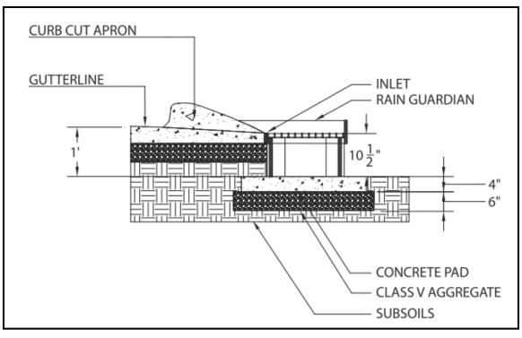
SLAB DIMENSIONS, DISTANCE FROM CURB, AND CHAMBER ELEVATION MAY VARY WITH SITE CONDITIONS. THE TOP OF THE METAL GRATE, HOWEVER, SHOULD BE 1.5" - 2" BELOW THE OVERFLOW ELEVATION AND THE CONCRETE SLAB SHOULD EXTEND WELL BEYOND THE FILTER WALL TO SERVE AS A SPLASH DISSIPATER.
