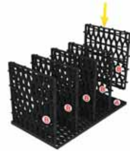
Fig. 13 Additional space for ports can be created by removing the center plate and moving the remaining internal plates toward the center (if possible).
