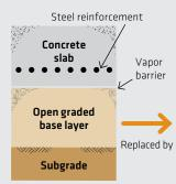
Drainage design featuring open graded base layer (OGBL)
